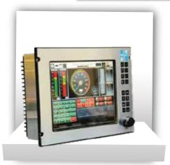
The Driver Display Unit (DDU) provides a man machine interface for the driver with a graphical mimic window in which various pre-defined screens to monitor major sub-systems of the locomotive or train.
