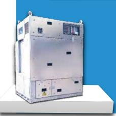
This energy efficient IGBT based 2x500KVA Hotel Load Converter installed in passenger locomotives, utilizes power from 25KV AC OHE to provide 750 V, 3-Phase 50 Hz supply required for feeding the electrical loads of passenger trains with up to 24 coaches.
