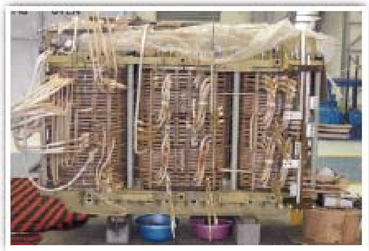
5400 KVA Loco Transformer Winding Assembly
